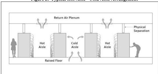
Figure 3. Typical Hot Aisle - Cold Aisle Arrangement
