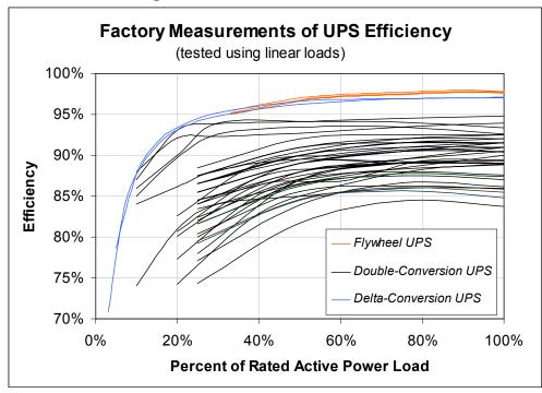
**Figure 4. Tested UPS Efficiencies**
